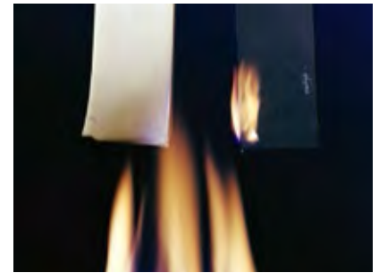
Flammability test Left: Silicone rubber Right: Organic rubber
